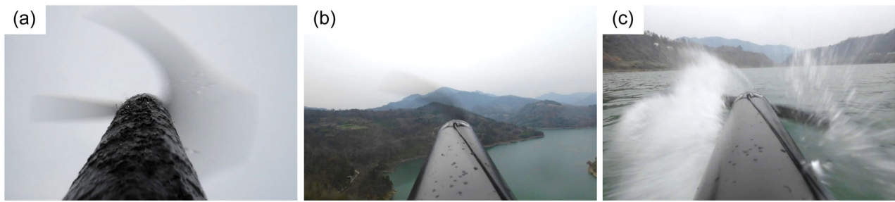
FIGURE 39 First-person view photo of the LB-II field test, (a) shows the moment LB-II emerged from the water, (b) shows the aerial flight phase, and (c) shows the moment of re-entry into the water. LB-II, Longbow II.
