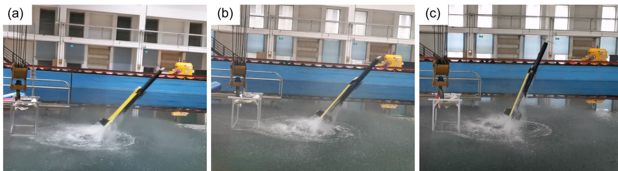
FIGURE 32 The pool water egress test in the pool with 0 m/s initial velocity and fixed initial pitch angle. (a) Initial angle of 70°, (b) initial angle of 75°, and (c) initial angle of 80°.
