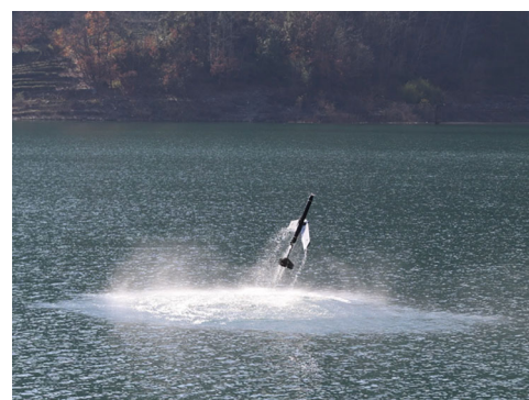
FIGURE 35 Longbow II flying upside down due to improper timing of wings deployment.
