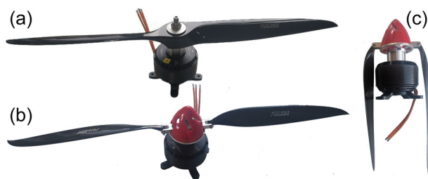
FIGURE 11 Different forms of air thrusters. (a) The 24 inch nonfolding propeller, (b) the 25 inch foldable propeller, and (c) the folded state of 25 in foldable propeller.
