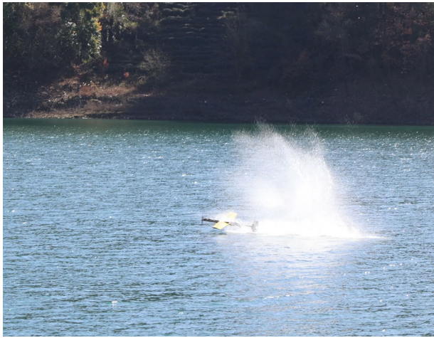
FIGURE 48 Longbow II bouncing up after entering the water and slamming the water surface.
