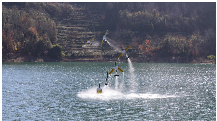
FIGURE 41 Synthesis diagram of Longbow II attitude changes during the water egress process.
